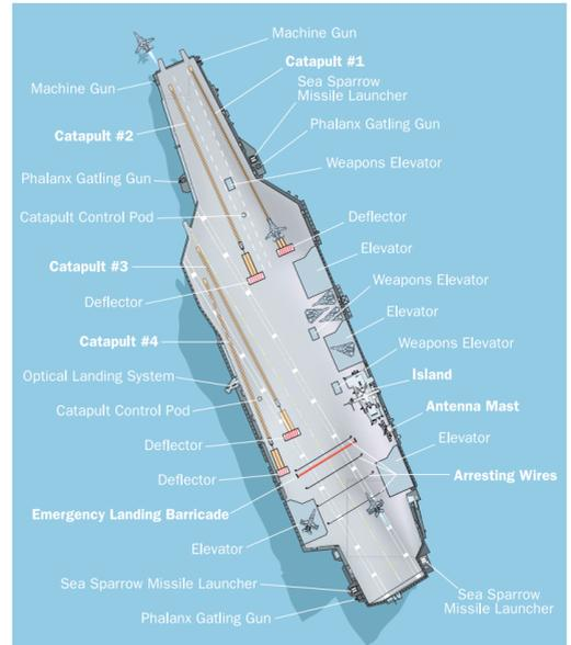
The diagram above shows how these various components fit together. Top View.
