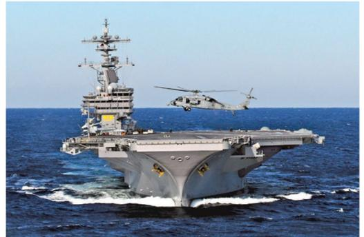
The aircraft carrier George H.W. Bush (CV-77) is the 10th and last of the Nimitz class of nuclear-powered supercarriers. The vessel is powered by two nuclear reactors that can operate for more than 20 years without refueling. The \$6.2 billion carrier is expected to serve as a Navy warship for about 50 years.
