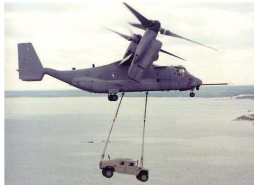
The Bell-Boeing MV-22 Osprey tiltrotor aircraft can haul up to 15,000 pounds of external cargo using dual hooks.
