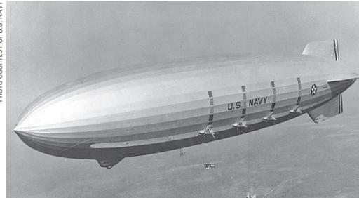
USS Macon airship recovering two F9C aircraft.
