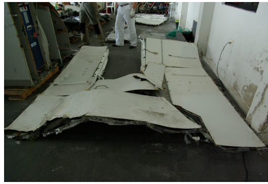
Figure 39: Ceiling of the LDMCR: with top-downwards deformation
