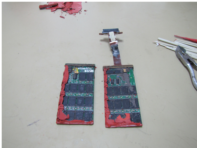
Figure 23: CVR memory boards before cleaning
