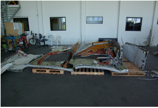
Figure 38: Floor of the LDMCR: with bottom-upwards deformation
